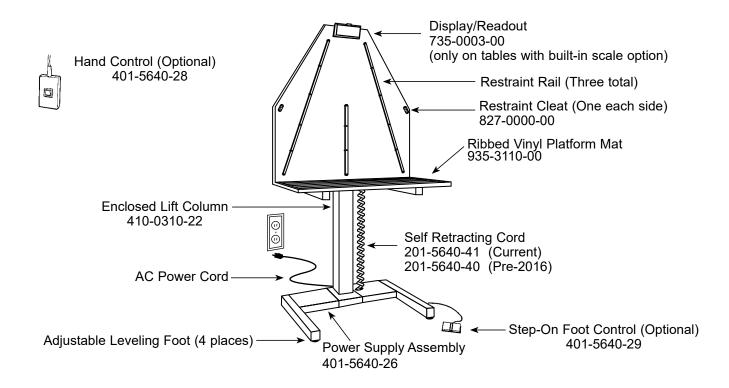
No. 101-5640-01 Electric Lift Exam Table with Hand Control No. 101-5640-07 Electric Lift Exam Table with Foot Control
